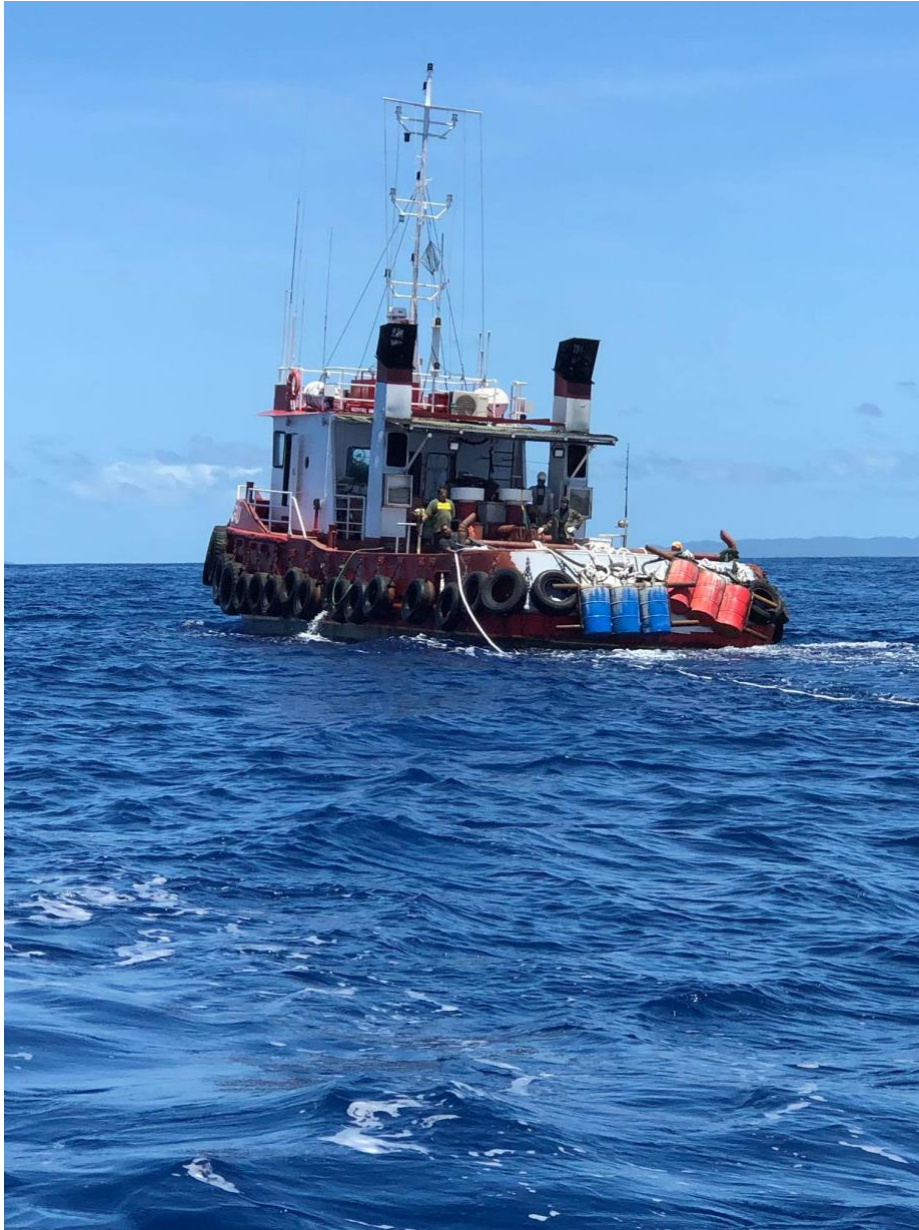
SSC Ksau deploys PSFA FAD – six oil barrels full of cement create the anchor. SSC Ksau has been deploying FAD's since 2007.
